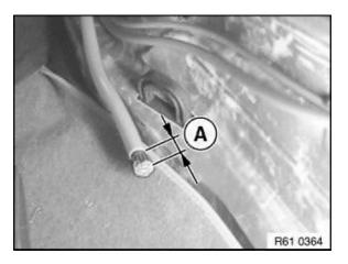
Strip insulation - length (A) - from cable end. Distance (A) = 15 mm.
