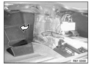
Release front side trim panel partly and fold forward.
