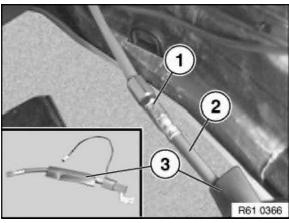
Push shrink-fit hose (3) over repair cable.
