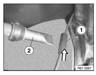
Push shrink-fit hose (1) over connection point and shrink-fit with a hot air blower (2).
