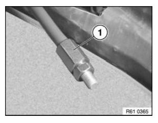
Push heavy-current connector (1) over stripped cable end and screw into position.
