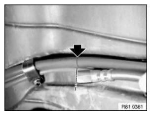
Lay repair cable parallel to battery positive lead.
