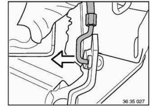
Press off locking washer (1). Disconnect pedal.
