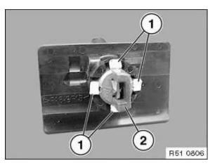
Insert vehicle key in lock cylinder (2).
