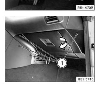
Close glove compartment cover. Lift out finisher strips (1) and unfasten screws. Remove glove
