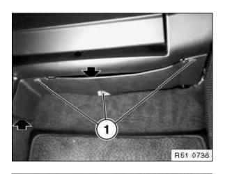
Release rotary clips (1) at bottom and lever out lower trim panel on left (risk of damage) and center.
