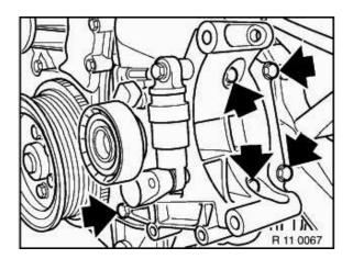
Remove mounting block for alternator.
